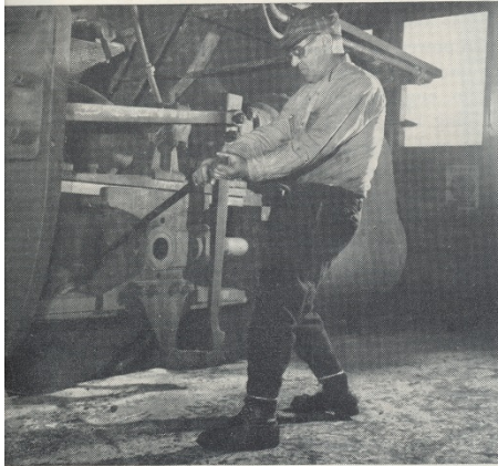
T. E. Berry sets crosshead and piston of an H-9s in proper position for blocking.
