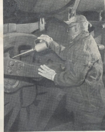
J. M. Douglas, at Philadelphia, oils driving box to ready steamer for last journey.
